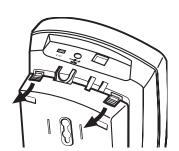
2. Plug one end of the supplied short modular cord into the phone jack on the back of the base.
